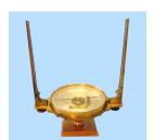
This is a one-of-a-kind size Gurley Mountain & Mining Vernier Compass especially built for both portability and sighting steep vertical angles. It was probably either a special order from the Gurley factory or a prototype of a new design considered by them but not put into production. The horizontal sighting arm is 9" long and the magnetic needle is 4 3/4" long. It has folding sight vanes that are an extraordinary 9 inches long. This length
