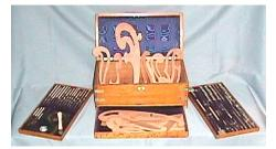
ivory handles of the pens. Over 90% of the items are original. There are 17 ruling pens plus 4 miscellaneous pens, a number of wooden triangles and French curves, and a brass protractor with measuring scale. The tools are contained in a hardwood case with three removable trays.
