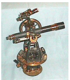
TR 20, Cradle-type Plain Theodolite , J.M. Hyde, Bristol, England, c. 1845.
