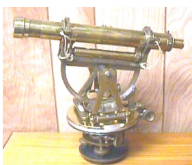
TR 20, Cradle-type Plain Theodolite , J.M. Hyde, Bristol, England, c. 1845.
