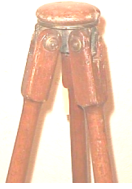
ET 15, Solid Leg Tripod , maker not indicated, c. 1890.
