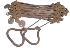
Gunter's Chain 33 Feet, 50 Links Iron Handles
