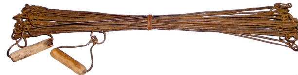
Two-Pole Chain 66 Feet, 32 Links Wooden Handles
