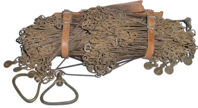
Metric Chain 50 Meters, 250 Links Brass Handles
