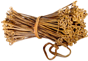
K&E Engineer's Chain 100 Feet, 100 Links Brass Handles
