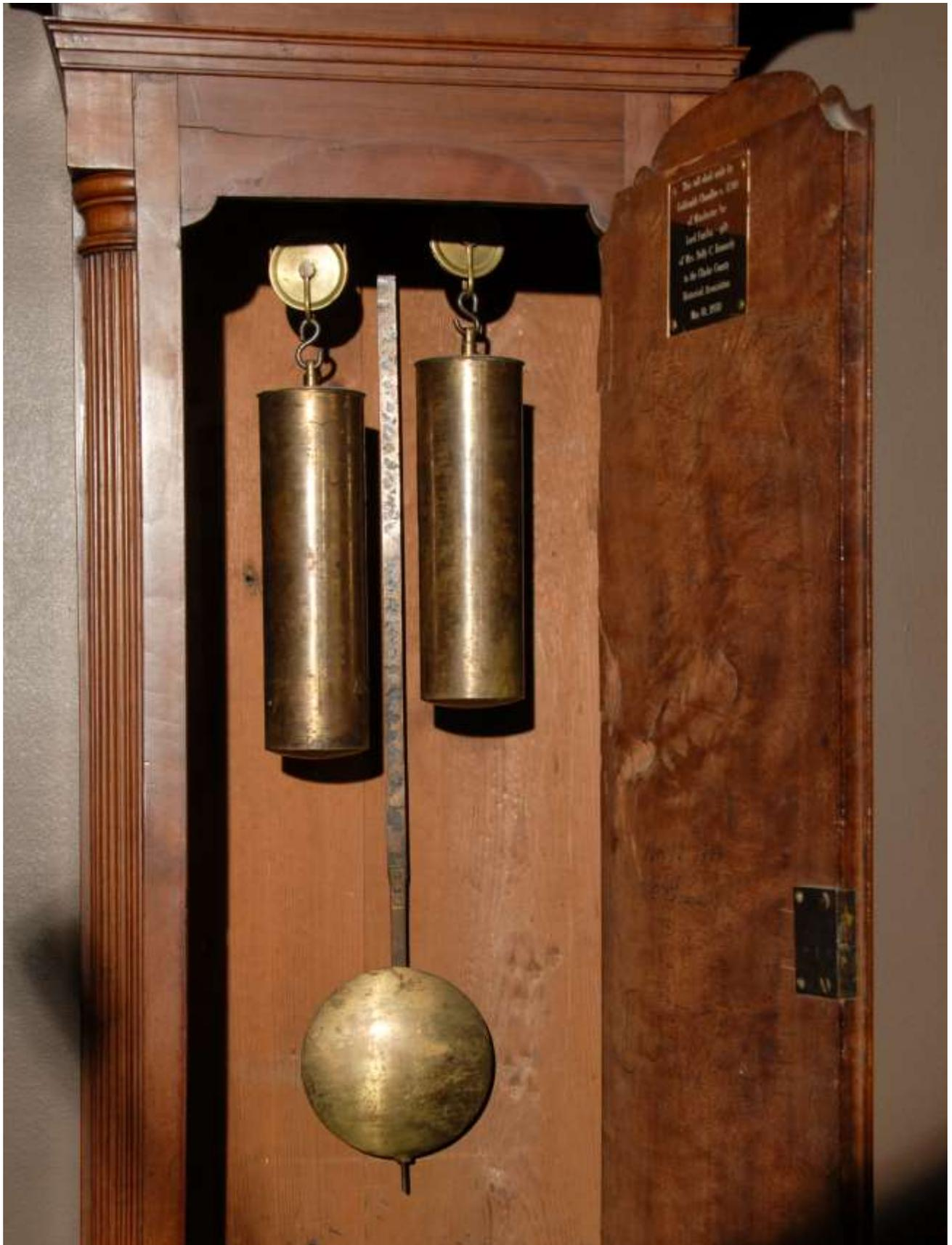
39 inch one second pendulum, Left weight hourly bell strike train, right weight for the time train, eight day clockworks by Chandlee
