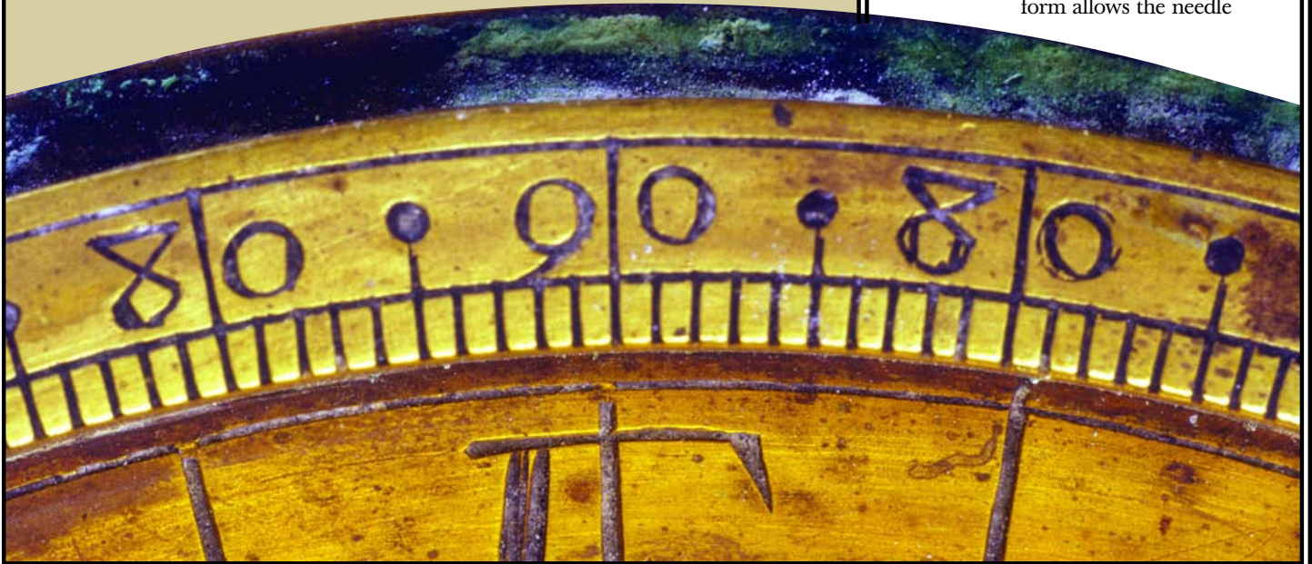
Figure 6 Final divisions inscribed with dividing knife Figure 7 (Below) Degrees on a signed colonial compass, dated 1733
