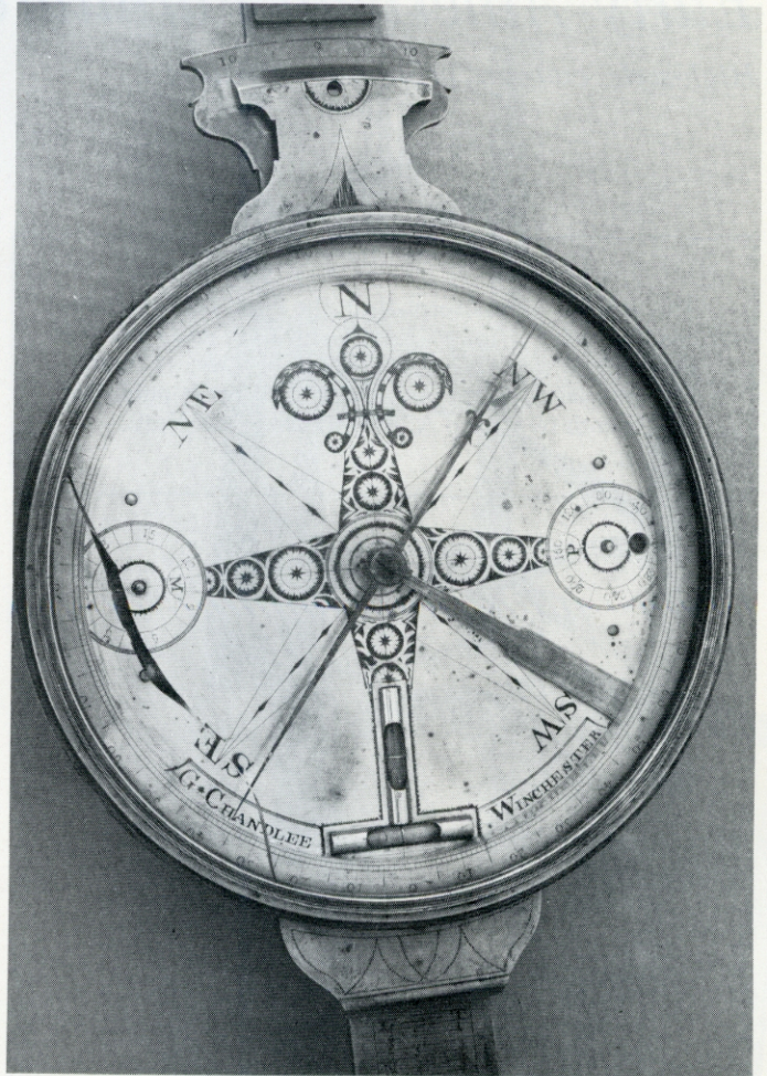
Fig. 11. Brass vernier compass, elaborately made and engraved by Goldsmith Chandlee, Winchester, Virginia (d. 1821), probably near the end of his life. The compass card is inscribed, G * Chandlee Winchester . The name A. Stowell Jr. is engraved on the brass cover. Diameter 7\frac{1}{8} inches.
