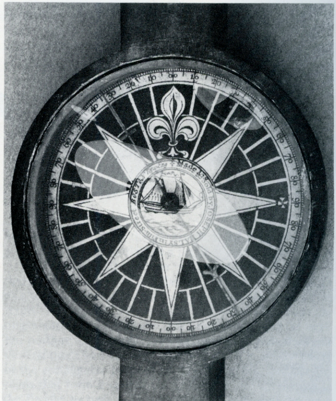
Fig. 1. Surveyor's compass made by Joseph Halsy, Boston, Massachusetts (d. 1762). Frame of apple wood with cherry cover inscribed, Richard Baxter his compass/bought Marche ye 2d anno 1747 . The engraved compass card has a medallion with a two-masted ship in the center surrounded by the inscription, Made & Sold by Joseph Halsy in Fish-Street Boston New Eng. Diameter 5¼ inches. All illustrations are from the collection of Pamela and Scott Guthman.
