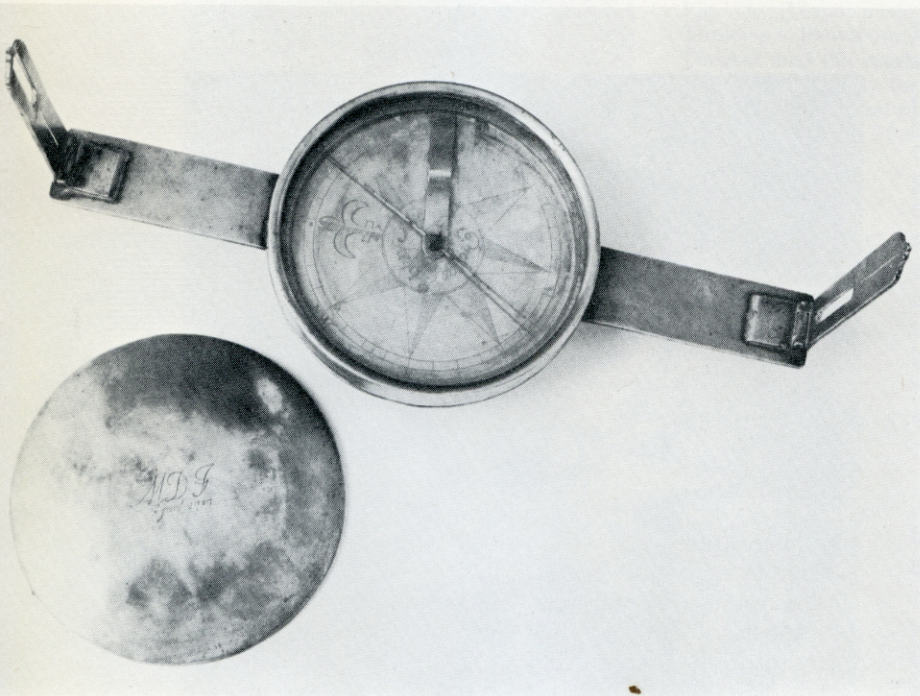
Fig. 4. Brass surveyor's compass made by John Avery, Preston, Connecticut. The cover is inscribed M D F/4th Jany 1787 . Diameter of compass, 5\frac{1}{2} inches.
