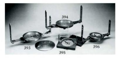
393. 5 1/4-Inch Plain Surveyor's Compass, c. 1815, "F.A. Heisely, Harrisburg (Pennsylvania)," 14" l. x 6 3/8" w. x 8 1/4" h. with detachable sight vanes, with brass cover, 2 vials (1 inset into compass face), silvered dial and outer ring, brass finish, with cutout fitted wooden case. \$1035
