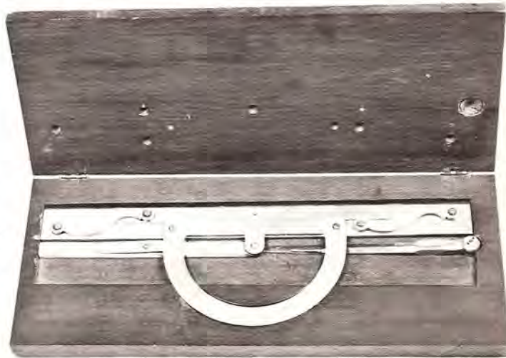
Parallel rule with protractor and plotting scale. Made for Henry Van Allen by Lebbeus Dod.
