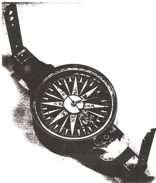
Vernier surveying compass made by James Doolittle of Hartford. Courtesy of the Chester County Historical Society's Museum, West Chester, Pennsylvania.
