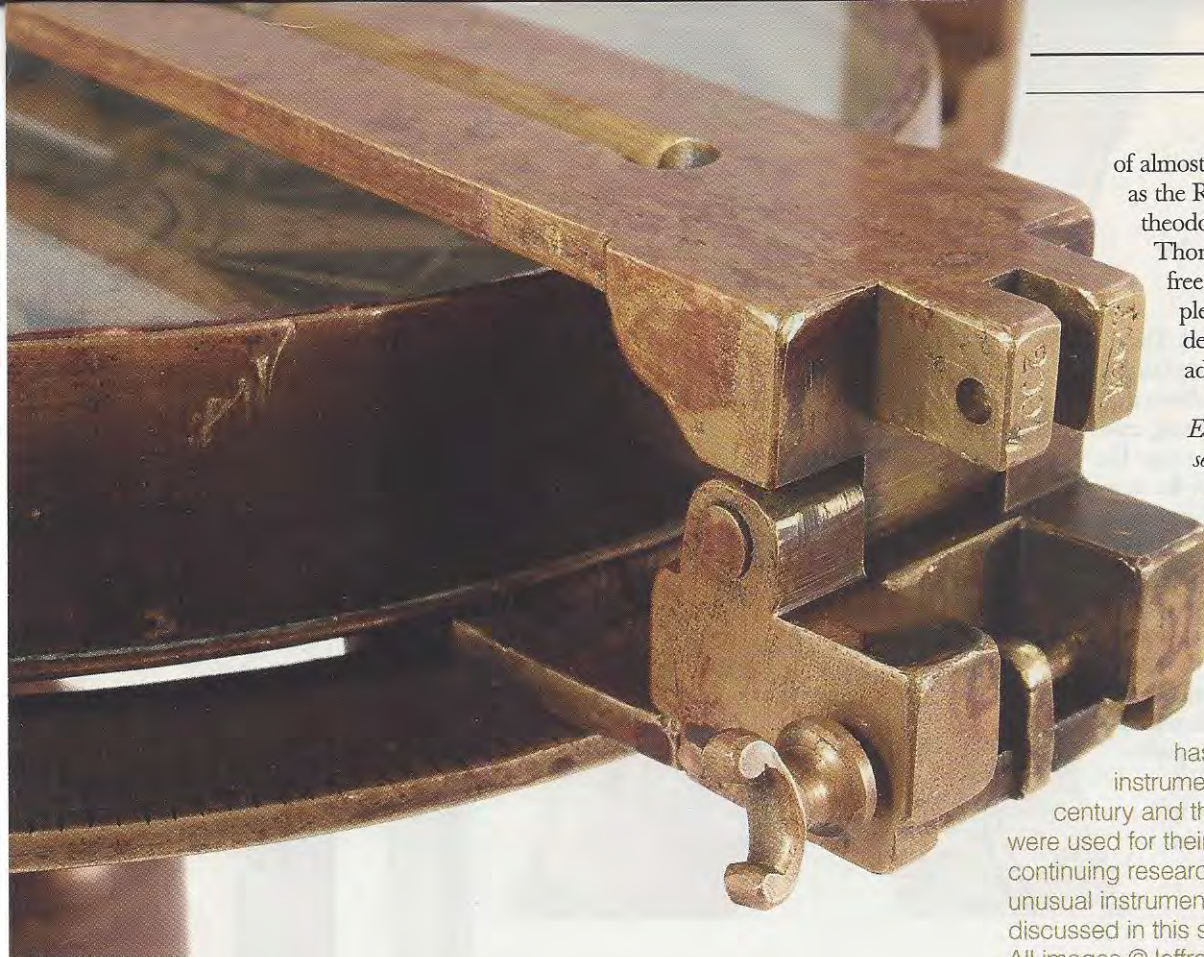
Figure 4 Restored folding sight vane assembly. (As in the case of responsible restoration, all of the replaced pieces on this instrument have been signed and dated so as not to provide any confusing historical data to future research. Under no circumstances should restoration affect the originality of existing pieces of an instrument.) Figure 5 (below) Detailed engraving on a Greenough circumferentor
