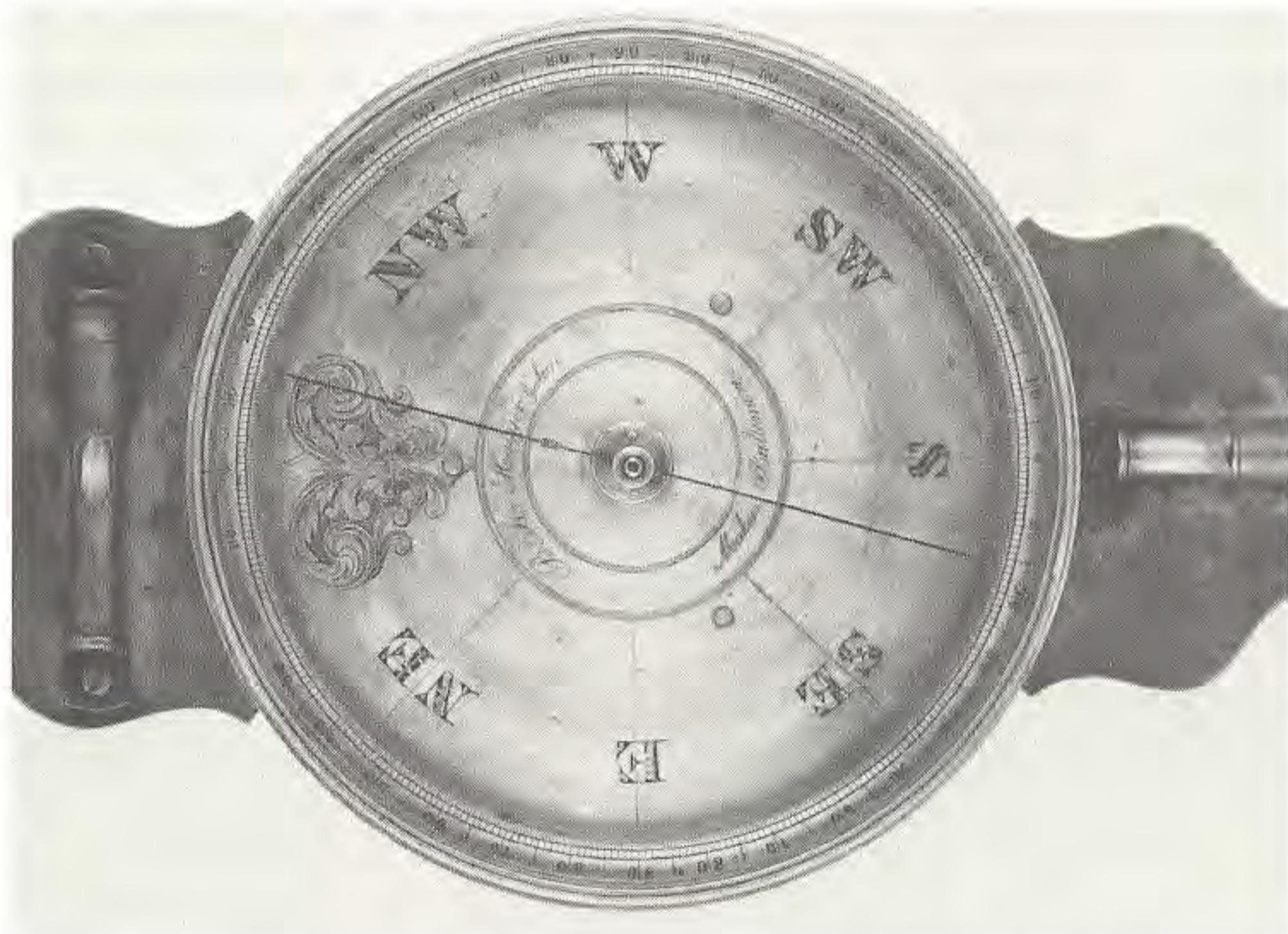
Surveyor's Plain Compass marked "B. K. Hagger & Son Makers, Baltimore" (NMAH--Gift of Baldwin-Wallace College)
