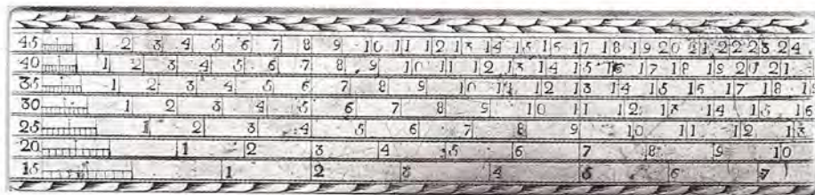
Brass plotting scale made by Benjamin Rittenhouse. Courtesy of the National Museum of American History, Smithsonian Institution.
