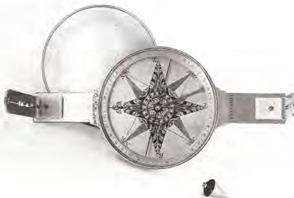
Plain surveying compass made by Benjamin Rittenhouse. Courtesy of the National Museum of American History, Smithsonian Institution.
