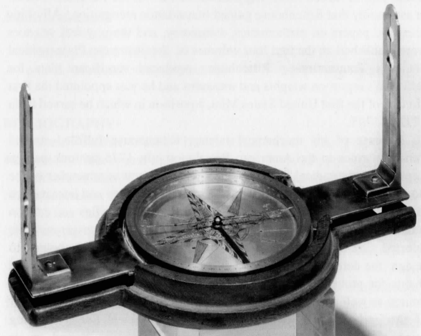
Fig. 7. Plain surveying compass made by David Rittenhouse and claimed to have been owned and used by George Washington after his retirement to Mount Vernon. Courtesy of the National Museum of American History, Smithsonian Institution.
