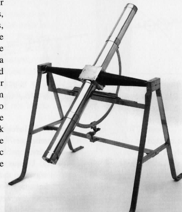
Fig. 3 Astronomical Transit Instrument built in 1769 by David Rittenhouse for his observations of the transits of Venus and of Mercury and later used it in his observatory at Norriton and later at Philadelphia. Courtesy of the American Philosophical Society.
