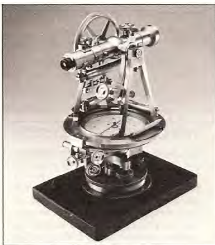
Aluminum surveying transit made by Keuffel & Esser of New York. It was taken to the North Pole by the American arctic explorer Commander Robert E. Peary (1856-1920) on his fourth voyage 1898-1902, during which he reached 87° 6' N., only 174 miles from the Pole, before he had to turn back. In the collections of the National Museum of History and Technology, Smithsonian Institution. (Photos courtesy of the Museum).
