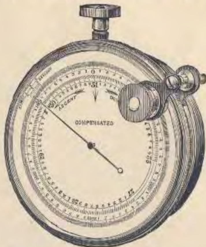
Special Surveying Aneroid Barometer
