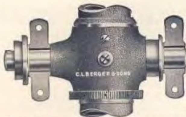
Cylindrical trunnions of the Berger Telescope Axis resting in their segmental wye bearings without strain. For adjusting the line of collimation, the telescope can be revolved 180° on its longitudinal axis.
