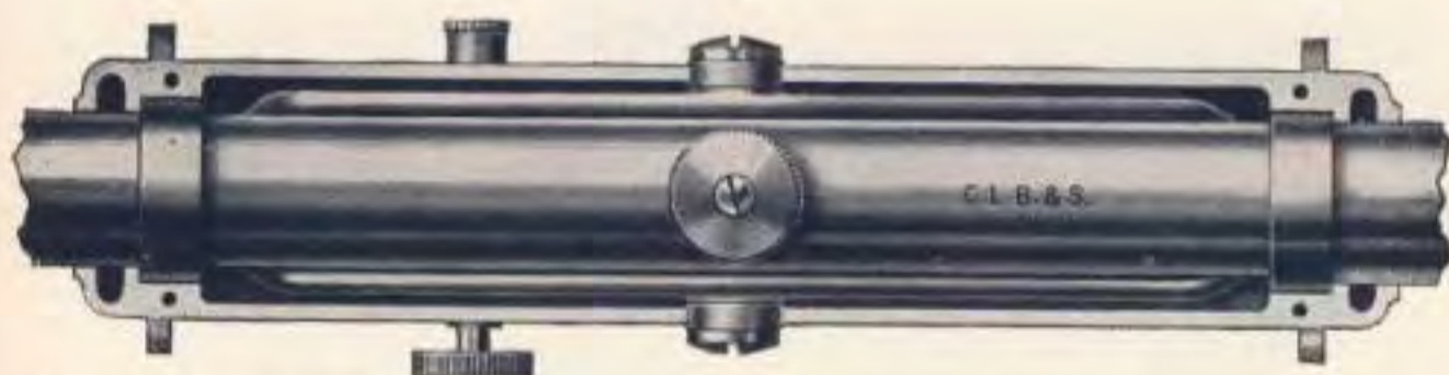
Plan view of Telescopes' Outer Housing and Center Bar (Cover Removed) The Collars of Telescope rest in 90° Segmental Wye Bearings of Housing Outer
