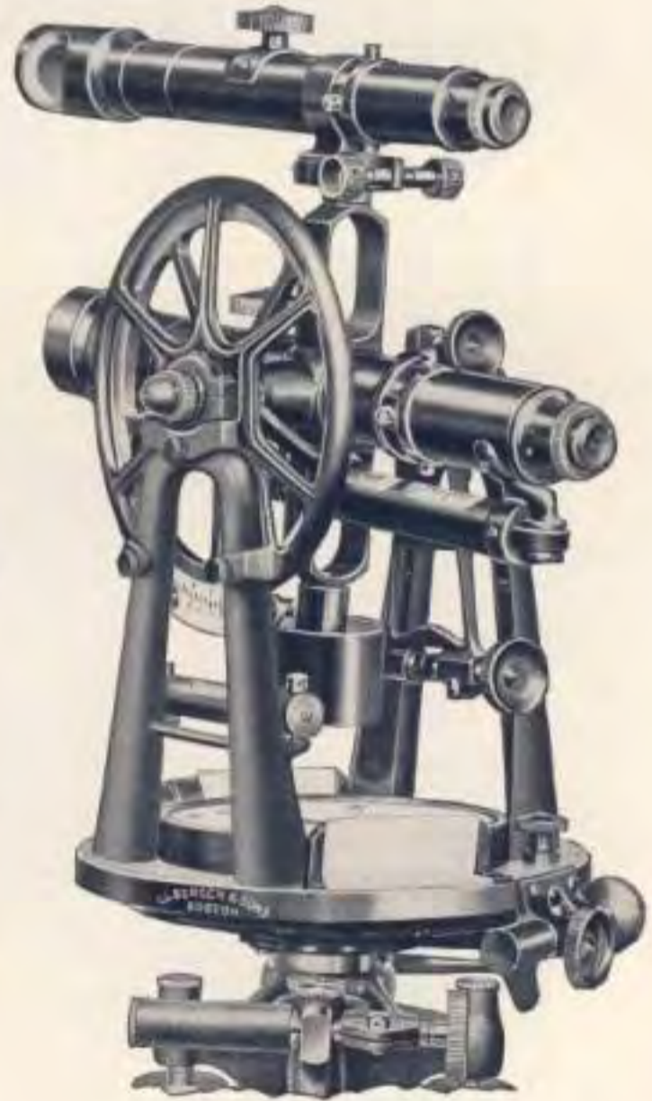
Auxiliary Telescope attached to the top of axis with counterpoise below for reading horizontal angles inaccessible with main telescope.
