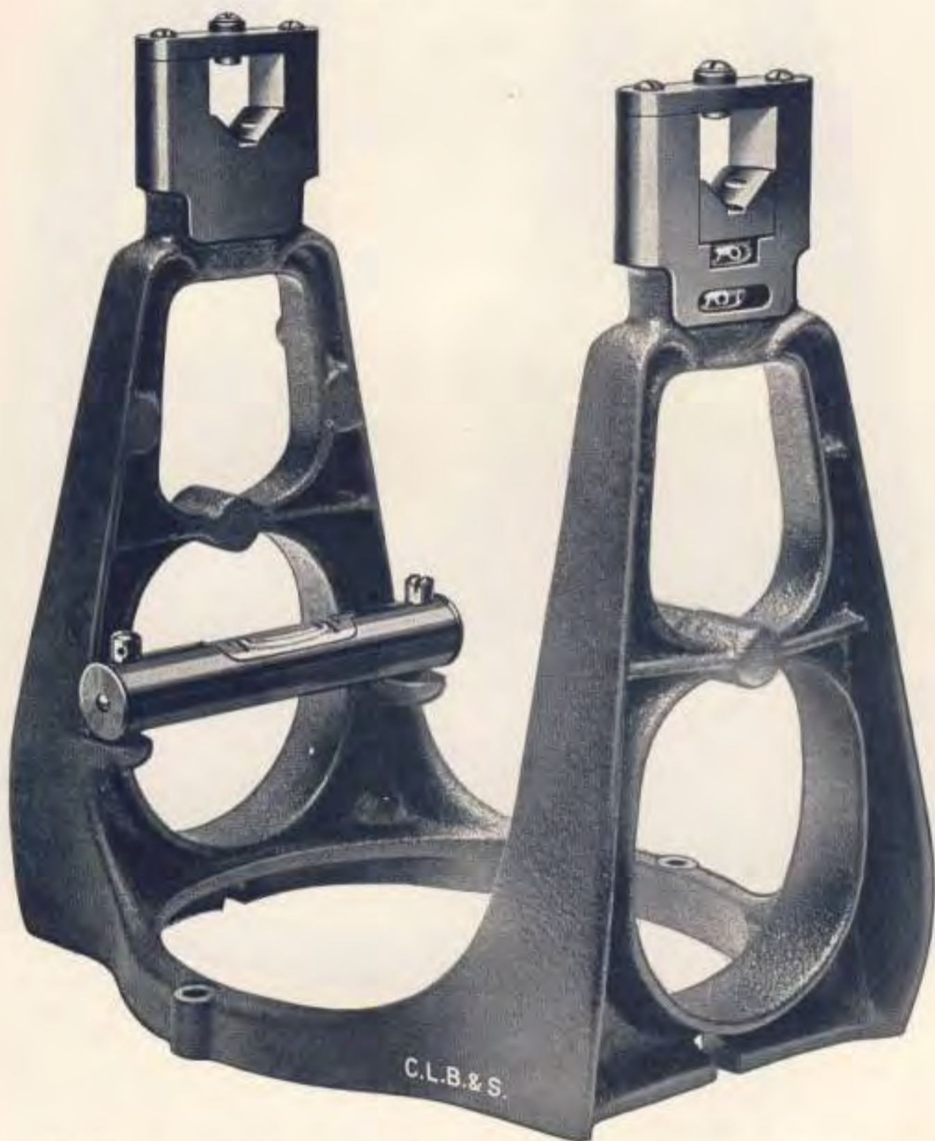
Cylindrical Trunnions of the Berger Telescope's Axis, resting in their segmental Wye Bearings without strain.
