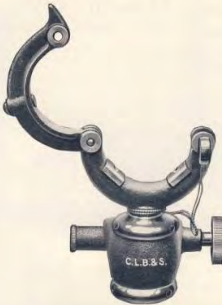
The bell metal collars of the Wye level telescope rest in 90° segmental wye bearings
