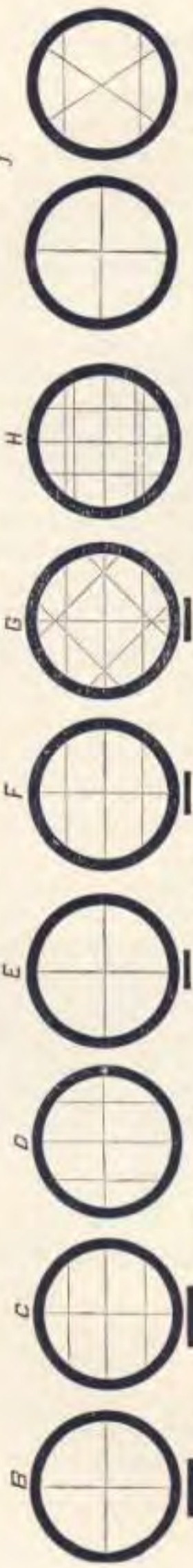
The Cross Wires for Dumpy and Wye Levels (Diaphragms C and D are provided with Stadia Wires)
