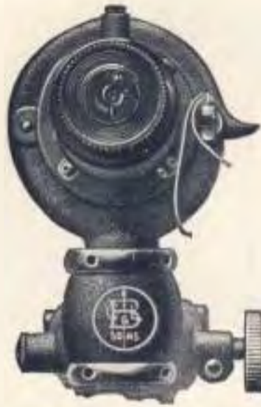
The Adjustable Wye is located at the Eye End of the Telescope
