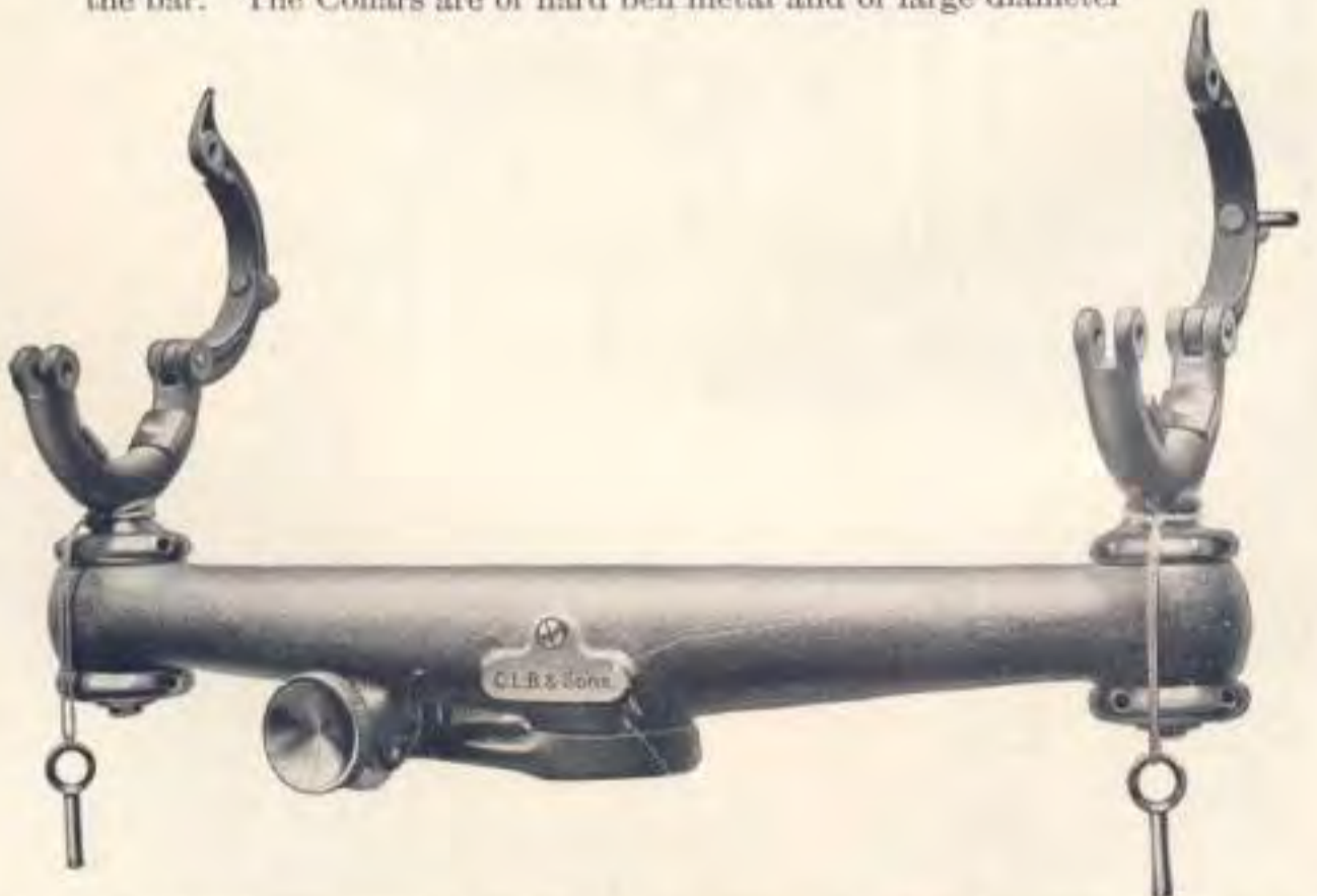
The Wye Stirrups open wide, which permits easy access, while reversing the telescope end for end, leaving the rest of the instrument undisturbed while making adjustments.
