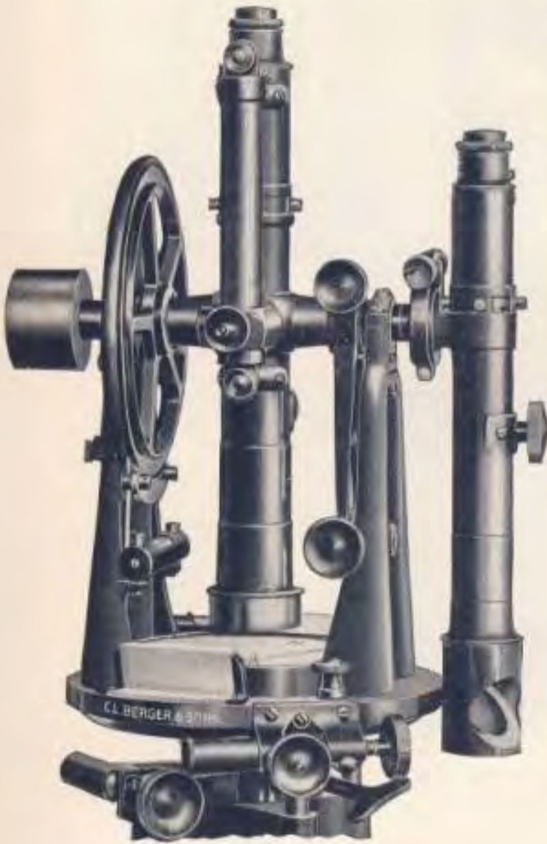
Auxiliary Telescope attached at side of axis with counterpoise opposite for reading vertical angles inaccessible with main telescope.
