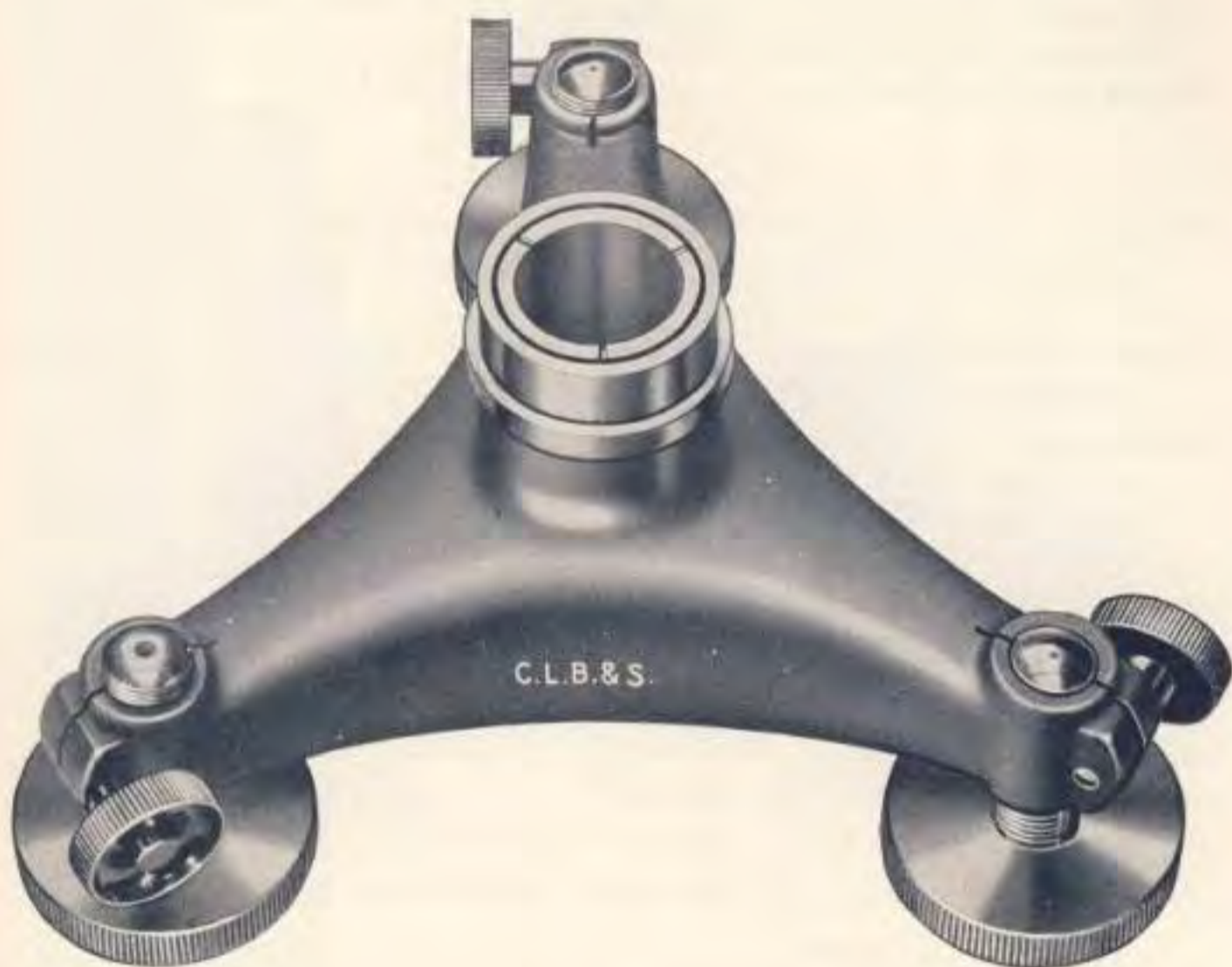
View of Three Screw Leveling Base, showing strain-proof Center Socket with very deep recess
