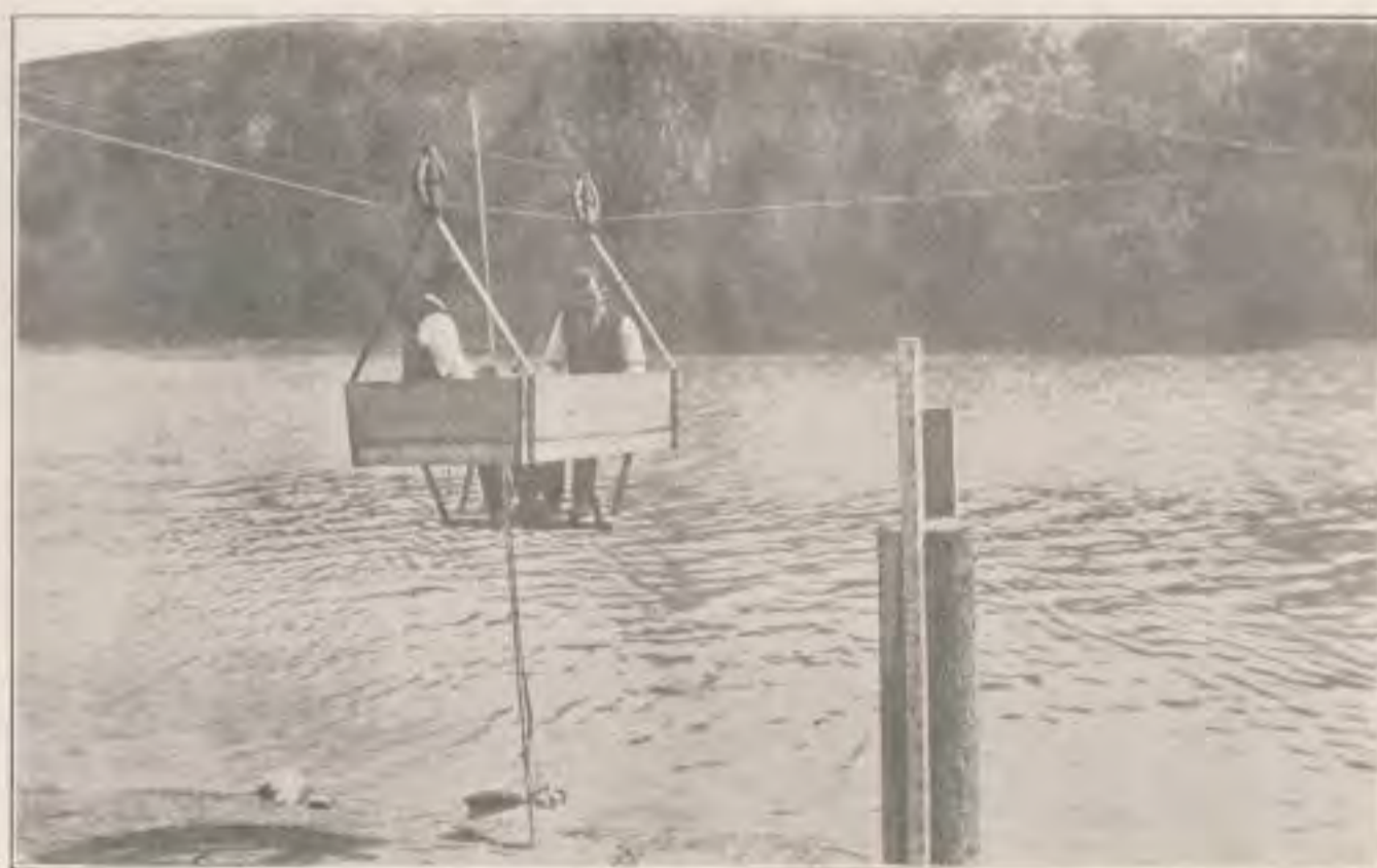
Canadian Government Engineers using a Gurley Current Meter suspended by jointed wading rod from a Cable Car
