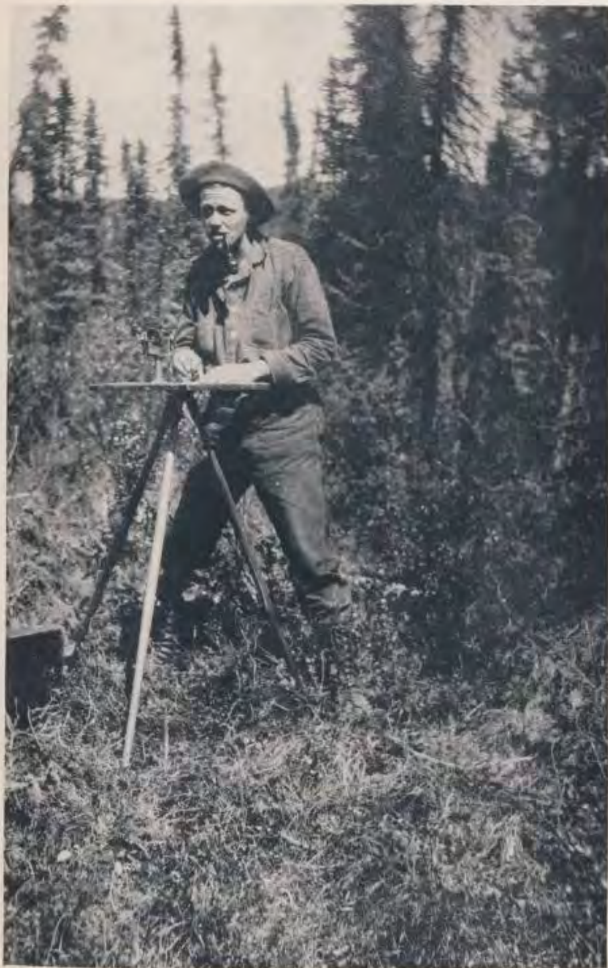
Traverseman of the International Boundary Commission using a Gurley Traverse Plane Table on Alaskan Boundary Maps
