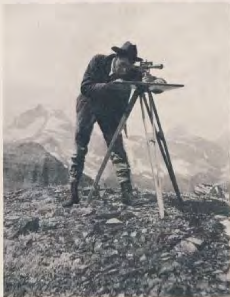
United States Government Topographers of the International Boundary Commission, at work with Gurley Plane Table Outfits. The upper view shows a station along the 141st Meridian, on the Alaskan Boundary Survey; the second view is along the 49th Parallel, at the Summit of the Rocky Mountains, on the United States and Canada Boundary Survey
