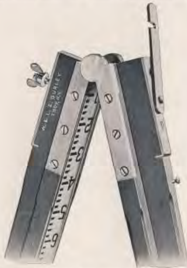
Enlarged View of Hinged Joint used on Rods Nos. 518-B, 519-B, 520-B and 521-B. Note the sturdy construction of the hinges and the manner in which the strong metal brace is anchored into the wooden rib; also the wing nut clamp screw.
