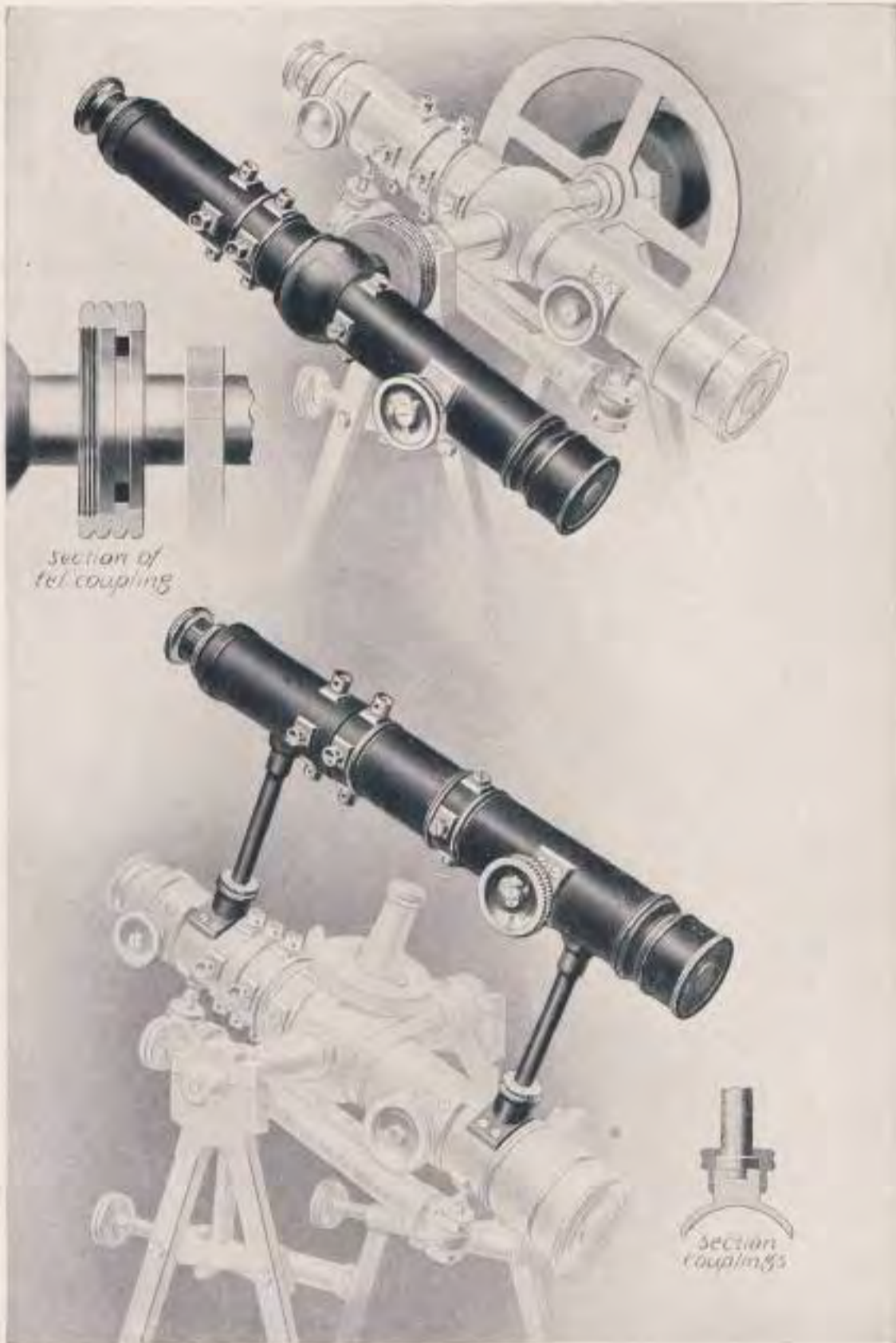
Nos. 160 and 161 Detachable Telescopes for vertical sighting in mine surveying. Each $33.00
