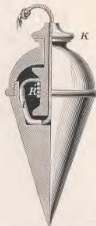
No. 465 Adjustable Plummet showing details of Concealed Reel
