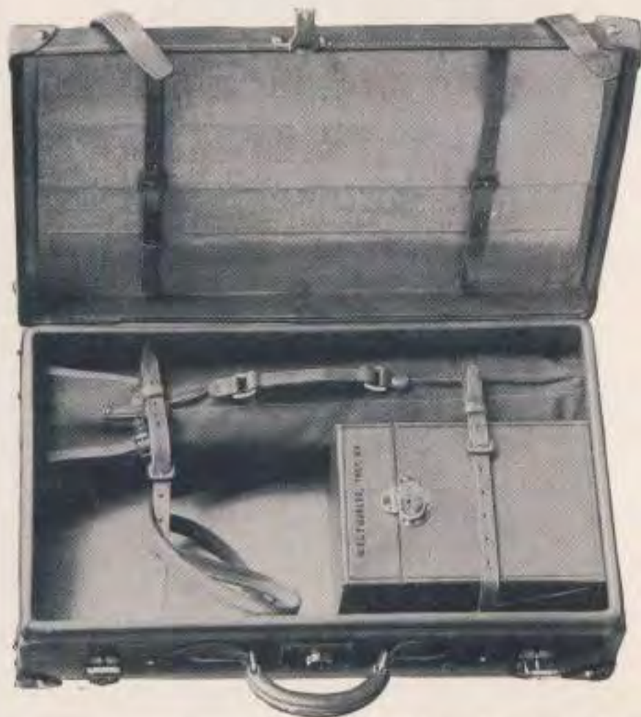
A Gurley Explorers Transit, with its special Tripod, packed in a dress suit case 24 inches long
