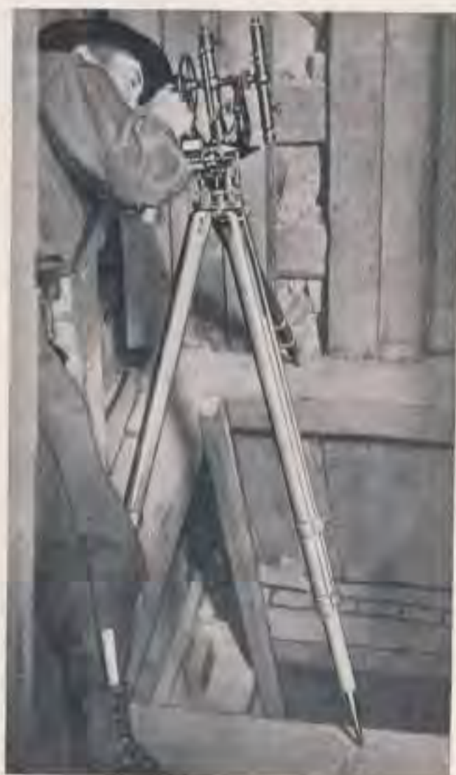
A Gurley Precise Transit equipped with Detachable Side Telescope No. 160. View shows instrument set up over a vertical mine shaft and observer using a magnifier to read the vertical limb
