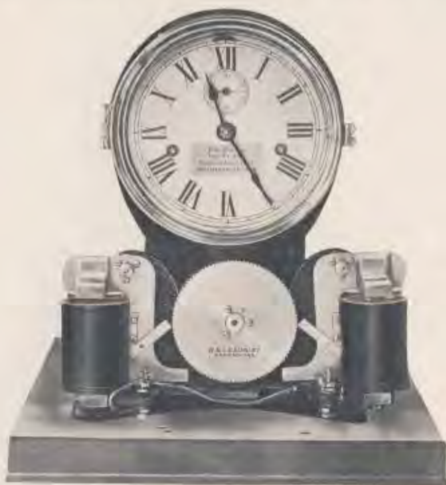
Long Distance Graphic Water Stage Register, showing the Receiver attachment
