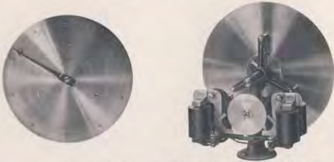
Front and rear views of Receiver with Indicating Dial, of the Long Distance Water Stage Indicator
