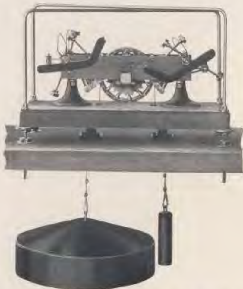
Float Operated Sender, for Long Distance Graphic Register
