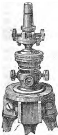
It also revolves upon the spindle as upon the ordinary compass ball, but can be clamped at pleasure to the spindle, and then by its sights or telescope directed precisely to any object by the tangent screw of the compound ball.
