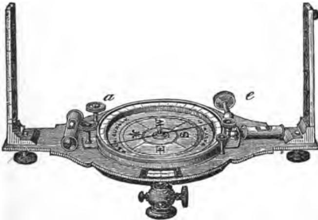
As shown in Fig. 10, this instrument has the main plate, levels, sights, and needle of the ordinary instrument, and has also underneath the main plate a divided circle or limb by which horizontal angles to single minutes can be taken independently of the needle.
