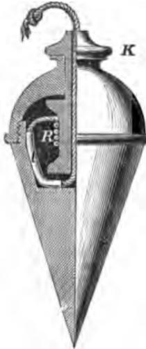
This plummet has a concealed reel, around which the string is wound by turning the milled head on top. The friction upon the reel within will hold the bob at any desired point of the line.
