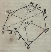
line from A, towards G, where let a peg be left, as at c; and again, the like distance from A, in a direct line towards B, where another peg is also to be left, as at d: let the distance from d to c be measured, and placed in the fieldbook, in the second column under the denomination of angles, in a line with station No. 1; and in the same line, under the title of dis-
