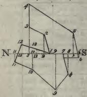
the point 2 raise a perpendicular to the eastward, the meridian distance being easterly, and upon it set 13.22, the second number in the column of meridian distances from 2 to 2, and draw the line 1, 2, for the first distance line : from 2 upon the first meridian, set the northing of the second stationary line, that is, 9.65 to 3, and on the point 3 erect a perpendi-
