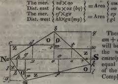
These four areas, am + ow + xp + glwill be the area of the whole figure cmswiprlc, which is equal to the area of the map abkm. Complete the fig.
