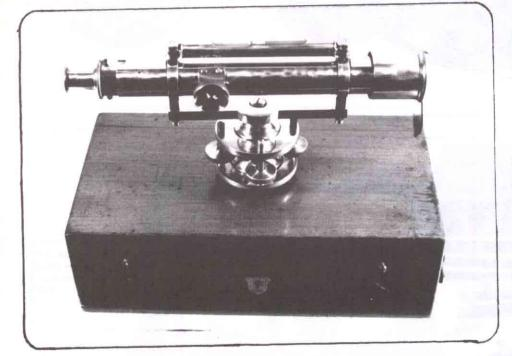
Su 85 DUMPY LEVEL, marked Sold by C. Baker, 244 High Holburn, London. Contains good 12" inside ratchet telescope with bubble mounted on top. Entire unit is highly polished brass, complete in mahogany case. 4-screw leveling.
