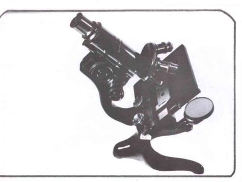
Mi547 MICROSCOPE by Ernst Leitz, Wetzlar. This is the finest working microscope we have offered. Horseshoe Base, Mirror, Shutter. Holder adjustable in two directions on stage. Mounts three lenses with one an oil immersion lens. Rack with course adjustment and micrometer adjustment. In beautiful condition with original lacquer on brass tube and fittings. Base is painted black. With carrying case and extra parts. A good old working microscope for the medical student today.
