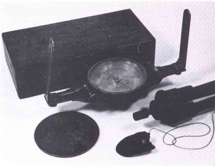
19. SURVEYOR'S VERNIER COMPASS WITH COMPLETE OUTFIT, circa 1845: Engraved on the compass is the maker; "Hewitt & Son...New York" a recorded instrument maker. The name was not in the city listing after 1853. What makes this instrument interesting is the unknown number of surviving compasses since the only reported one was privately owned in Connecticut. The compass is 5 3/4" fully hand-engraved and overall 15 3/4" with engraved vernier. The outfit has a brass cover, ball and socket joint, plum, tripod, and case. A very old mend of brass secures one arm and bubble levels are complete. Other examples are unknown....$725.
