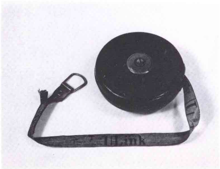
23. LEATHER BOUND SURVEYOR'S TAPE MARKED WITH LINKS: A 19th. century cased measuring tape made specifically for surveying use. The case is 4" with brass rewind knob and trim. The tape itself is 50' long, showing some use and marked by links . Made by "Chesterman" these were imported for American surveyors with inches on the reverse of the link marks....$75.
