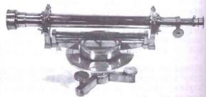
This is one of the most unusual forms of the little known "Egault's Level" (somewhat favored in France) that we have ever seen. It has a compass and azimuth scale (which the conventional Egault Level does not) and is obviously a hand made item. Much of it is filed out of stock brass. The underside of the compass shows a trial (and faulty) engraving of the inner dial. There has been so little Mexican instrument making that this instrument is an important find.
