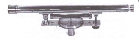
18. EXCEPTIONAL TROUGHTON LEVEL - English, late 18th c, signed "Troughton/London". Bright brass with original lacquer finish 98% intact (mostly minor pinpoint spotting), telescope 21" long, 14" d fixed focus objective, draw tube focusing of eyepiece upon cross hairs, 7" bubble level above 44" d compass with silvered face, 3 3/8" needle, signed on 104" long base, 5 3/4" overall ht. Missing protec-
