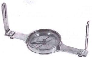
116. WELL MADE SURVEYOR'S COMPASS - English, 1st qtr 19th c, c, signed "Spencer & Company/LONDON". Bright brass, base 12 3/4" long, screw-on sight vanes 5 1/8" h, compass 4 7/8" d with silvered face, 3 3/4" needle, 6 1/2" overall ht. Staff clamping screw lost, otherwise very fine overall condition. No case.
