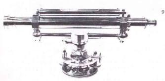
99. ELEGANT SURVEYOR'S LEVEL - American, 3rd qtr 19th c, unsigned. Bright brass 15 3/4" long, 7" h inc1'd 4-screw leveling base, 8" level bubble. Focussing by eyepiece draw tube. Original dovetailed mahogany case with front doors 18" w, 6 1/4" deep, 8 3/4" h. Case in good to very good, level in very fine condition.
