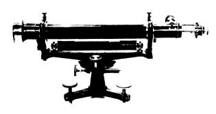
This instrument of French design is an unusual combination of wye and Dumpy levels. The bubble level is attached to the frame (can be adjusted) while the telescope by itself can be reversed in the wyes, one of which is screw adjustable. The 3-screw base permits its use on a plane table with a screw hole for tripod mounting. This form of instrument is virtually unknown in our country.
