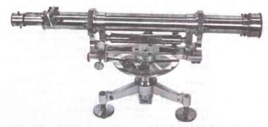
152. THE MOST SPECTACULAR WYE LEVEL WE HAVE EVER HAD - German, probably c. 1900, signed "C. Luttig in Berlin". Bright brass, original lacquer finish, standing 11" h incl 3 screw leveling tripod stand, telescope 20" long with 1 5/8" d clear aperture objective and 6 1/4" bubble level. Azimuth readout to 30 arcseconds by opposing verniers on silver scale inlet into 6 1/4" d bearing plate. Each vernier is fitted with its own magnifier. Original dovetailed oak case 22" long, 10" w, 12" h. Case
