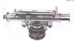
167. FINE COMPACT LEVEL - English, c. 1850, signed "Troughton & Simms, London". Bright brass, original lacquer finish except on repaired sunshade where it has been restored, 6 1/2" h overall including 4-screw leveling base.
