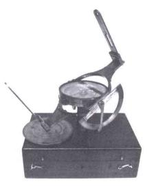
WAGON WHEEL PENDULUM-ODOMETER, American, late 19th century, signed, "Keuffel & Esser Co., New York". A leather-covered cylindrical container 5" in diameter, holds a heavy double-dialed pendulum-counter and frame. The outer dial records from 0-100 revolutions, and the inner dial, read directly through a window in the outer dial,
