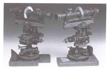
enables measurements by chain accurate to 1/10,000 of a foot. Edward H. Holden was the Engineer in charge of surveying in the Bronx Burroughs of New York. He designed these instruments for accurate traversing in city streets, bridges and tunnels. We believe that few of these instruments were produced. K&E discontinued advertising the Holden instruments by 1921. These are impressive and extraordinary American-designed high-precision instruments...\$2200 pr.
