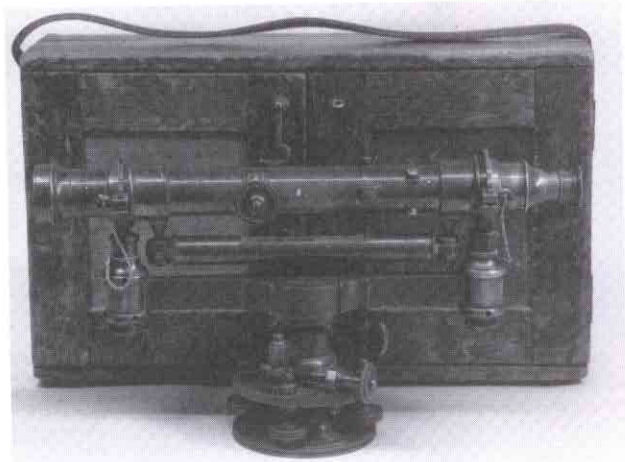
32. BOSTON WYE LEVEL , late 2nd quarter 19th century, nicely signed, " C.G. King, Boston ". This early American wye level is 14 1/2" in length and incorporates a 7" long barrel bubble, an early style directly-threaded slow-motion tangent screw, and a 4 screw leveling base. The top of the supporting frame is decoratively engraved with the manufacturers name and a 5 point star. The condition of this heavily-built Instrument is good. The original double door case is in fair condition....$675
