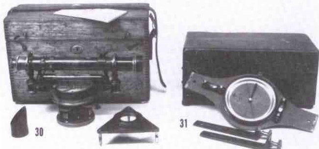
30. K & E ARCHITECTS LEVEL/COMPASS , American, 1906, signed, " Keuffel & Esser Co. New York ". This small level includes a telescope 11 1/4" in length, a housed compass with 2 7/8" needle, a horizontal circle with opposed vernier, and leveling base. The set also includes a wall trivet and points, two adjustment pins, lens cover and shade, and a later booklet on the use of the instrument. The condition is very good; the case is sound but stained....$395 31. PHILADELPHIA PLANE COMPASS , American, late 19th, early 20th century, signed by engraved script, " Queen & Co. Makers Phila. 5945. ". This small plane compass is 11 3/4" in length and includes a 4" long needle, opposed level vials and 5 3/4" tall sight vanes. The condition of the instrument is very fine, complete with 99% of the original finish throughout, and complete with the original case....$595
