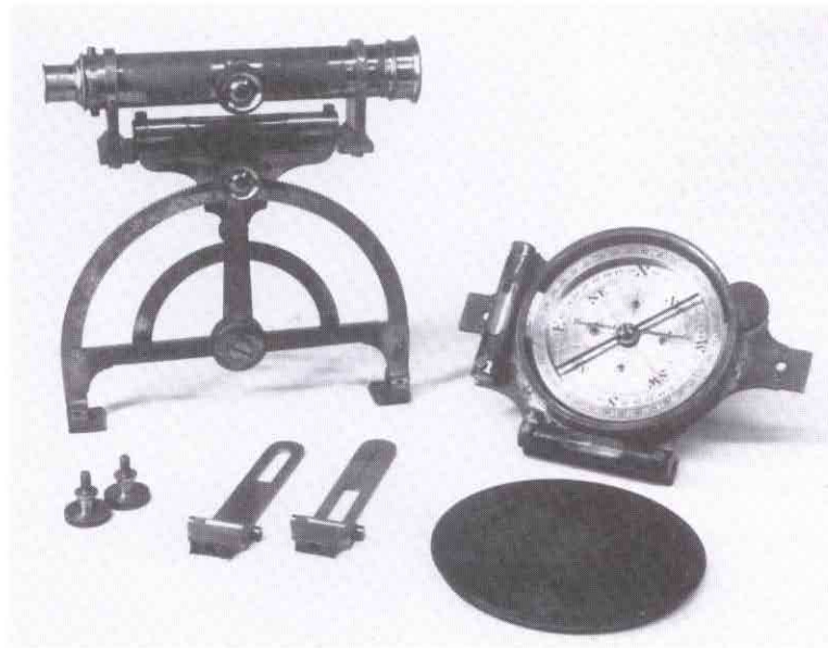
15. PRISMATIC COMPASS , American, mid-late 19th century. This Hutchinson pattern compass is 2 3/4" in diameter with a single folding sight vane and fold-up prism with a swing-away cover. It is in fine condition and is complete with its velvet lined leather case.....$225
